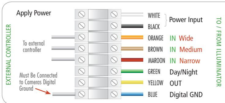
To activate desired angle the corresponding output on the external controller must be set to active low.
