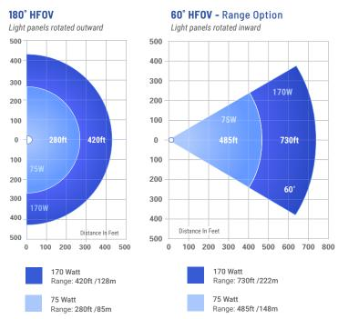
Light Panels can be rotated by increments to achieve coverage in-between these ranges.
