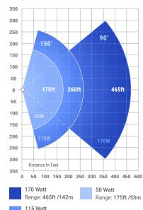
Light Panels can be rotated by increments to achieve coverage in-between these ranges.
